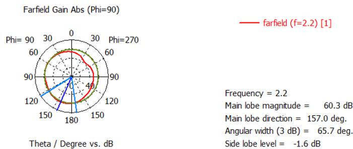
**Figure 3:  $\epsilon_r = 2.2$  Multi Substrate with Rect. Patch and  $h=1.6$  mm and Frequency=2.2GHz, Gain = 60.3**
