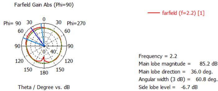
**Figure 2:  $\epsilon_r = 2.2$  Single Substrate with Rect. Patch and  $h=1.6$  mm and Frequency=2.2GHz, Gain = 85.2**
