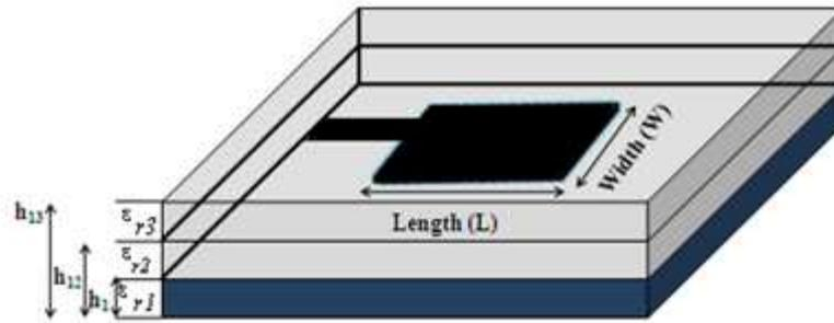
**Figure 1: Multi Layer Microstrip Patch Antenna**
