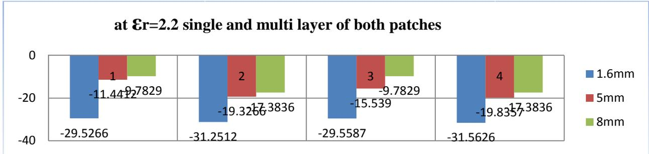
Figure 4:  $\epsilon_r = 2.2$  Comparison of Return Losses for Both Patches
